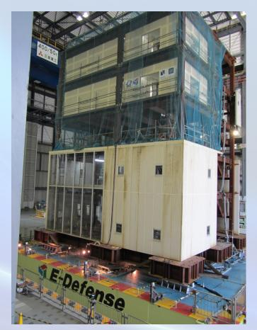
Five-story test on base isolation and nonstructural systems at Japan's E-Defense shake table facility during August 2011
